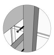
Drive the screw in predrilled hole
