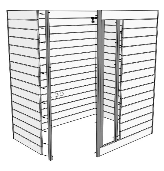
1. Install the door and window frame brackets in the locations indicated on the original plan.
